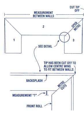
(P) You will notice that the last wing does not go all the way into place. Put it as far into place as possible keeping the miter cuts perfectly aligned. Measure the distance (?) as indicated in the example. Divide this dimension by 2.
